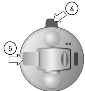
\* Pull the antenna out until firm resistance is felt. The antenna will extend to 25.5cm.
