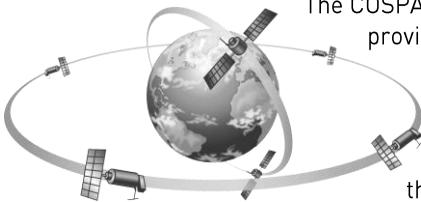
The COSPAS/SARSAT system utilises two satellite arrays to provide distress alert and location data to search and rescue authorities. The GEOSAR system can provide near immediate alerting within the coverage of the receiving satellite. The LEOSAR system provides coverage of the polar region beyond the range of the GEOSAR system. It can calculate the location of
